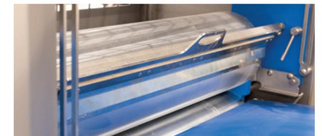
*Wear resistant roller scrapers to keep the rollers of the reduction stations as clean as possible*
