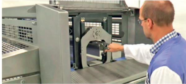
*Efficient, error free operation and tool change-over is realized by applying Unique Fit Tooling. Because of the lightweight and more compact tooling, handling and detaching the tools is as easy as possible and can be done by one person. No other devices are needed to help the operator change the tools.*
