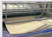
3. Laminating: to obtain a finer and more regular cell-structure and a stronger dough.
