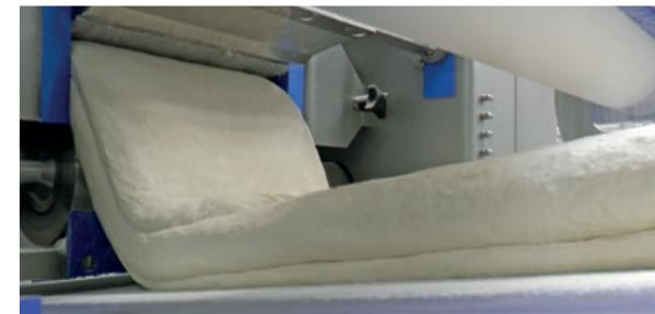
*Elimination of falling heights: by minimizing the transportation height throughout the production line, it results in a stable and relaxed dough sheet.*
