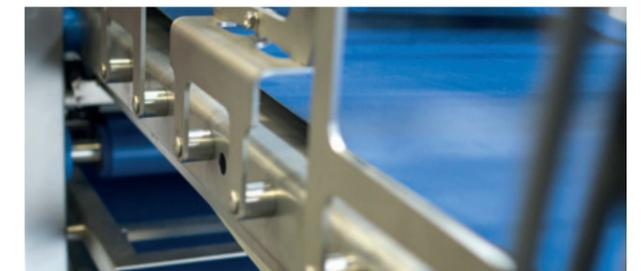
*Accumulation of dirt and dust is reduced due to the application of stand-offs.*
