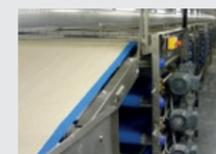
7. Proofing: the dough sheet or products can be proofed, depending on the type of products and production process.
