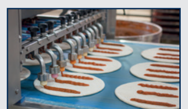
5. Sauce depositing: Tomato sauce is deposited on the pizza base. Various methods are available, for instance showerhead depositing and stripe depositing.
