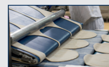
5. Dough recycling: the rework dough is transported back to the pre-sheeter. This brings our Pizza Base line to a highly effective and cost saving level.
